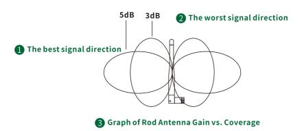
According to the transmission characteristics of the antenna to the signal, in order to ensure the optimal image transmission effect of the wireless suit, it is required:
