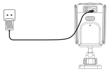
Please charge the Battery Camera with the included power adapter for at least 5 hours.
