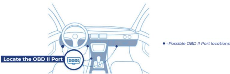
OBD II Port locations are different depending on the type of vehicle. Above are the most common locations.
