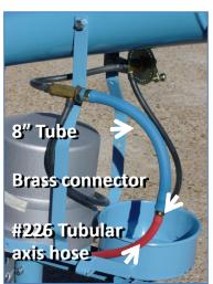
10. Connect to 8" Tube: Connect the remaining 8 inch rubber tube from the needle valve (#701) (or stuffer valve for Model M-8) to the tubular axis hose (#226) with the supplied
