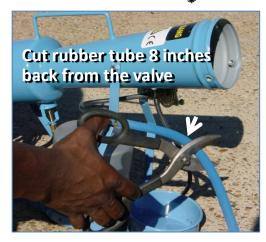
5. Rubber Tube from Needle or Stuffer Valve: Cut the rubber tube 8 inches back from needle valve on Models M-3 and M-4, and 8 inches back from stuffer valve on Model M-8. The 8" tube will be connected to the tubular axis hose in Step 10.
