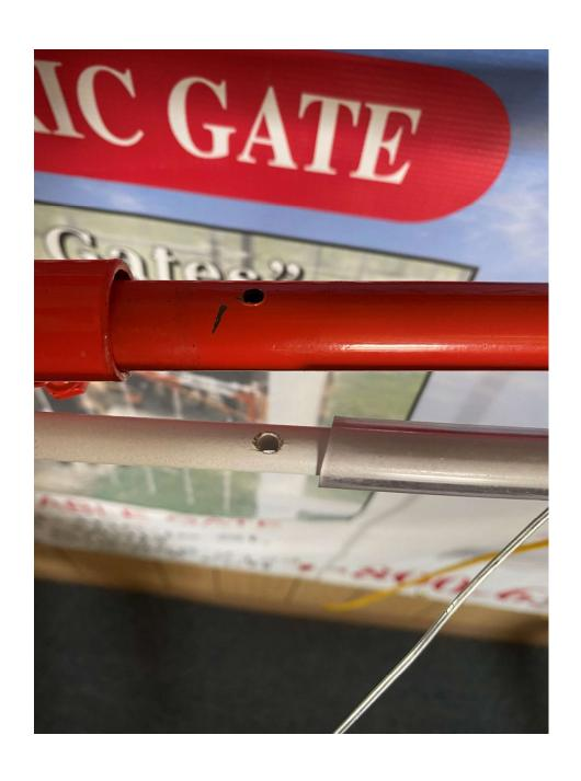
Insert the fiberglass rod with hose w/streamer in to the telescoping section assuring the holes line up. Secure with a cotter pin from the bottom. Weave the electricity carrying wire through the welded half chain link on the end of the telescoping section. It is designed to break away if it gets caught on equipment.
