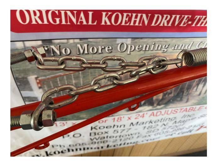
Hook other end of spring to the chain link that is welded on top of the main frame.
