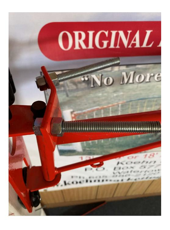
Use the hex nuts to fasten each side of the chain to the ends of the adjusting bolts. Hook up one end of the spring on to the middle link of the chain.
