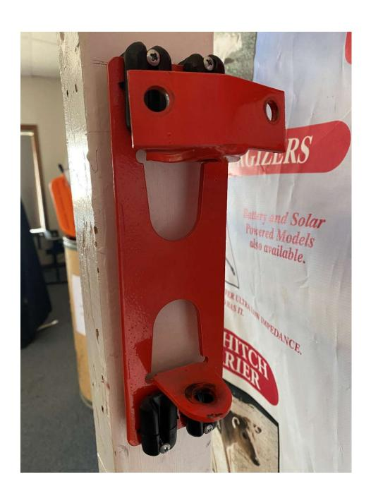
Install the main frame by dropping the 1/2" pin through the hinge plate and the main frame. Secure it by putting a cotter pin in the pre-drilled hole in the 1/2" pin.
