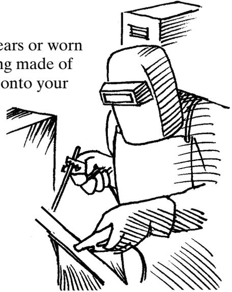
**Always wear the proper protective clothing for welding.**
