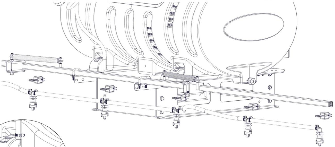
Loosely slide a hose clamp on to the feeder hose, connect the boom feeder hose to the hose barb tee on the nozzle harness and secure with the hose clamp.
