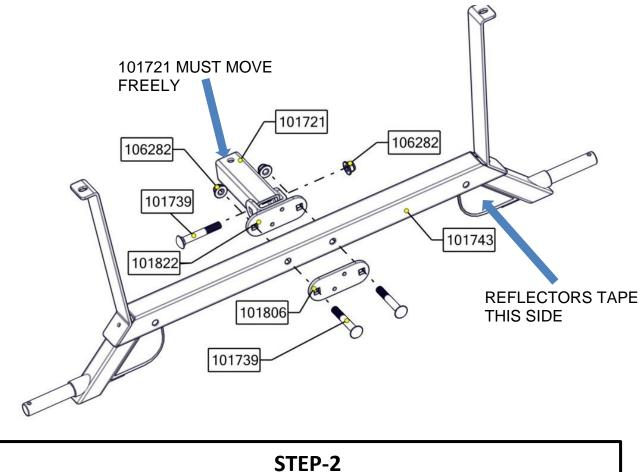
1. USE ASSEMBLY FROM STEP-1 AND ASSEMBLE TO (102238) TONGUE ASSEMBLY WITH FASTENERS AS SHOWN. **DO NOT OVERTIGHTEN**, MUST MOVE FREELY
