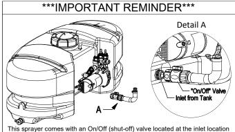
of the tank, towards the underside. (See Detail A). You must make sure the valve is in the "open" position before using your sprayer.
