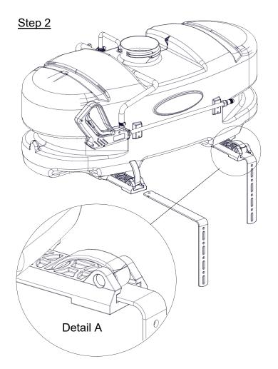
After your tank brackets are securely attached, turn the tank assembly over and position it so that the cam handles which extend beyond the back of the tank are facing you and just hanging over the edge of the table or flat surface you are assembling this on.
