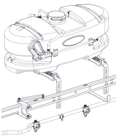
With the boom secured to the boom mounting brackets, the nozzle harness can now be attached.
