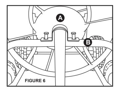
7. Using the 1.75" bolts (J), insert them thru the bushing and thru the holes on the frame (B). Attach lock nuts. Repeat for other side of the spool. After the 4 bolts and nuts are attached you may tighten the nuts.
