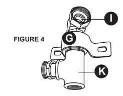
Screw the galvanized tee (K) onto the spool end
