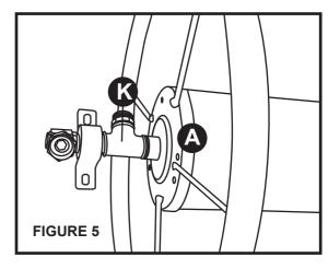
6. Place the spool **(A)** on the frame **(B)** so the bushings are oriented over the holes on the frame. You may have to compress the spring to get the spool oriented properly.
