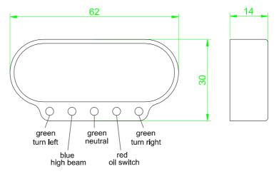
As a option the right turn control lamp can be used for a additional warning function which will provide a +12V signal. To connect both sides of turn signals together to the left turn control lamp the please refer as the schematic below.
