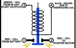
When 12V+ is applied to terminal 3 the trigger coil a magnetic field is generated, lifting the trigger to close the circuit between terminal 1 and terminal 2 and activating the starter motor.
