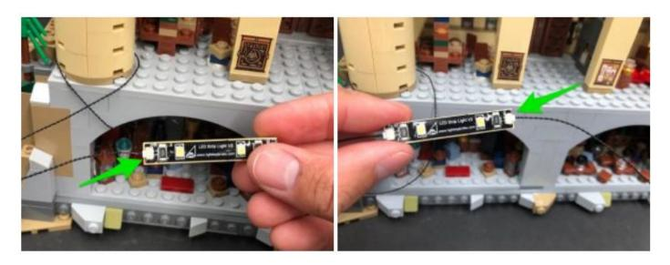
Thread the other end of the 15cm connecting cable up and over the following brick along the ceiling of the hall then mount the strip light to the hall ceiling above the library as shown below:
