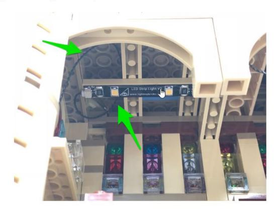
Thread the other end of the 15cm Connecting Cable through and over the next brick on the ceiling then pull it out from the other side and connect it to left port on the remaining **White Strip Light** stuck onto a **provided LEGO Plate 1×6**.
