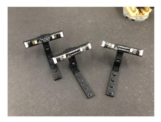
**67.)** Take a **RGB 30cm Connecting Cable** and connect one end to the left port on one of the ground spot lights. Connect the other end of the cable to the left port on one of the upper spot lights.
