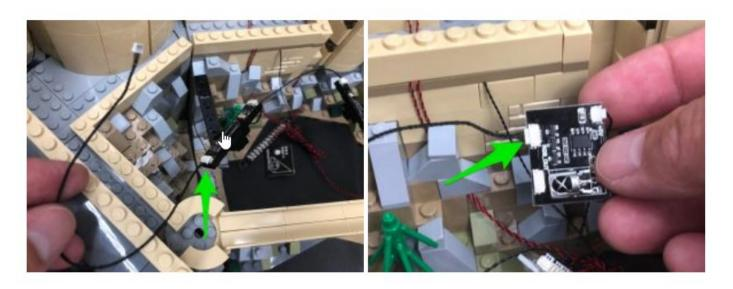
Lastly, ensure the RGB Board is facing the correct way up so that the IR sensor is visible and in line of sight to the remote control we will use to control it.
