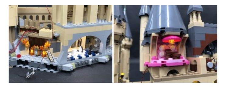
**50.)** Neatly tuck in the cables, effects board and two expansion boards inside the back left side of the mirror of erised room.
