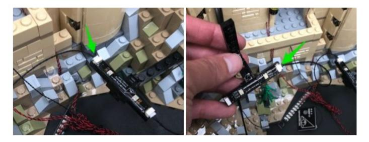
Connect the spot light to the below position to allow it to project up onto the large main tower of the castle.
