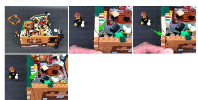
9.) Connect both Bit Light cables to spare ports on the 6-Port Expansion Board, then turn ON the battery pack to test the Service sign lights are working OK.
