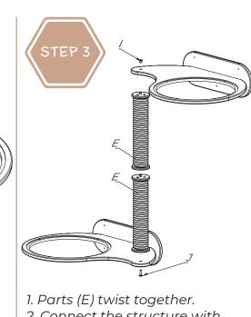
1. Parts (E) twist together. 2. Connect the structure with the products using screw (J) and nut (I).
