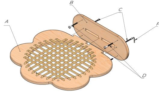
The panel A is installed in the groove of the part B, then it is screwed with the confirmations C using the key F.
