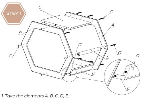
2. Fasten the parts with screws (F) and (G) as shown in the illustration using a hex wrench (H).
