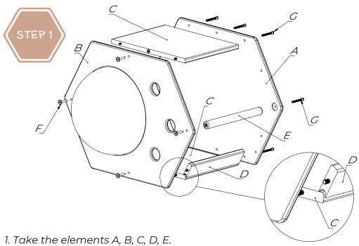
2. Fasten the parts with screws (F) and (G) as shown in the illustration using a hex wrench (H).
