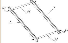
1. Take the elements H, I, J. 2. Fasten the parts with screws (M) as shown in the illustration using a hex wrench (P).
