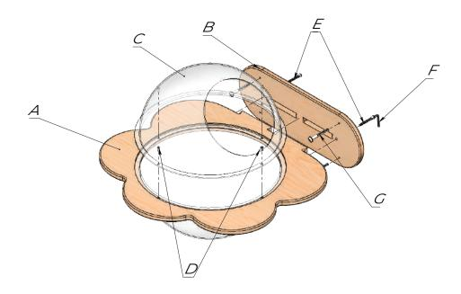
The panel A is installed in the groove of the part B, then it is screwed with the confirmations E using the key F. We install the upper cover C on the part A and fix it with the help of screws D.
