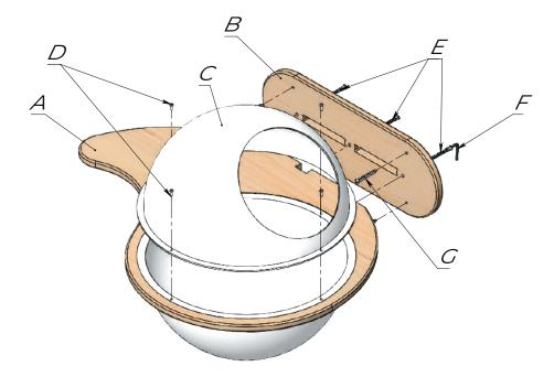
The panel A is installed in the groove of the part B, then it is screwed with the confirmations E using the key F. We install the upper cover C on the part A and fix it with the help of screws D.
