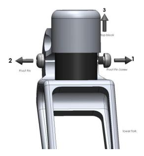
**Step 3.** Attach Frog Leg caster fork to wheelchair by insert the original stembolt and washer from the bottom up through the Frog Legs top block and into the receiver on the wheelchair as shown in Illustration #1. **IMPORTANT: Make sure to align the teeth of the camber washer to match the original angle.**
