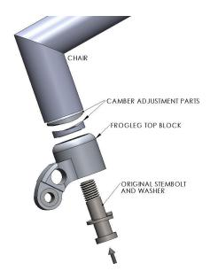
**Step 4.** Make sure that the polymer dampener is placed coin side up in the machined seat (a hole that does not go all the way through) in both blocks. Re-assemble the two sections (top and bottom) of the Frog Leg shock absorbing caster fork. *NOTE: Your Frog Leg suspension forks are designed with a slight pre-load so the forks may have to be pressed against a solid surface in order to line up the holes.* Tighten the pivot pin with the 4mm Allen wrenches. See illustration below.
