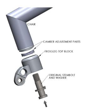
NOTE: Before removing the existing rigid caster forks it is important that you note the angle of the adjustment camber so that this position can be duplicated with the new Frog Legs suspension fork. In order to help you maintain the camber, we recommend that you remove/install the forks one at a time so that the installer can refer to the other camber position.
