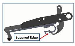
If your TiLite clamp looks like the clamp to the left, with a squared edge at the bottom, you will need to either replace it with Part P102 or use a Dremel and remove material and curve the bottom (see picture on right).
