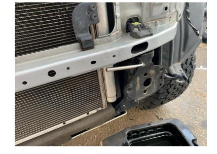
\*Installation of this hardline can be tricky with the KDSS models. Patience while passing the hardline through the rad support will help a lot at this step
