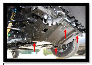
Remove 4 bolts and factory front Skidplate.
