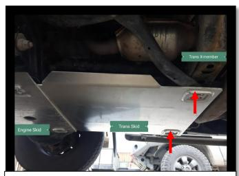
Remove 4 factory bolts from support bars. Install OKX Transmission Skid as shown, placing slotted spacers between Skid and support bar tabs.
