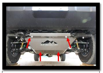
4. Install OKX Engine Skid using 2 factory bolts and supplied M8x35mm bolts, washers & 3/8" spacers.
