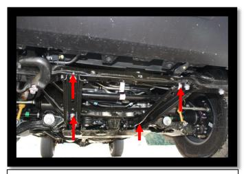
3. Remove Skid support brackets, save 2 factory bolts for installation of OKX Engine Skid.
