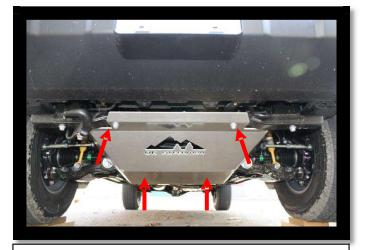
4. Install OKX Engine Skid using 2 factory bolts and supplied M8x35mm bolts, washers & 3/8" spacers.
