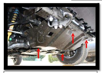
Remove 4 bolts and factory front Skidplate.
