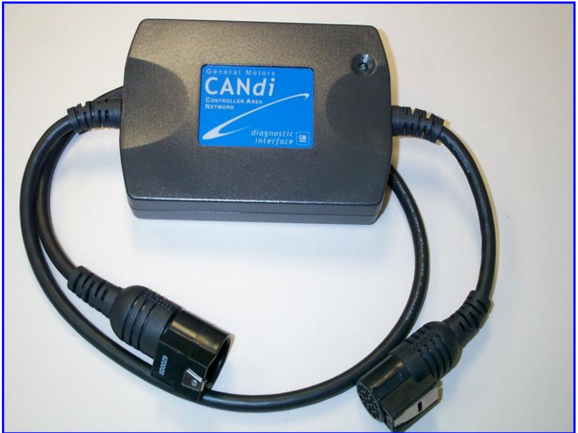
Controller Area Network diagnostic interface (CANdi) module
