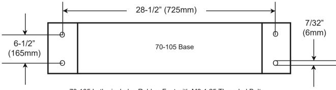
70-105 Lathe includes Rubber Feet with M8-1.25 Threaded Bolts
