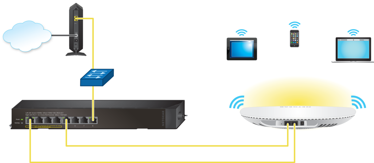
Figure 8. Link aggregation connection
