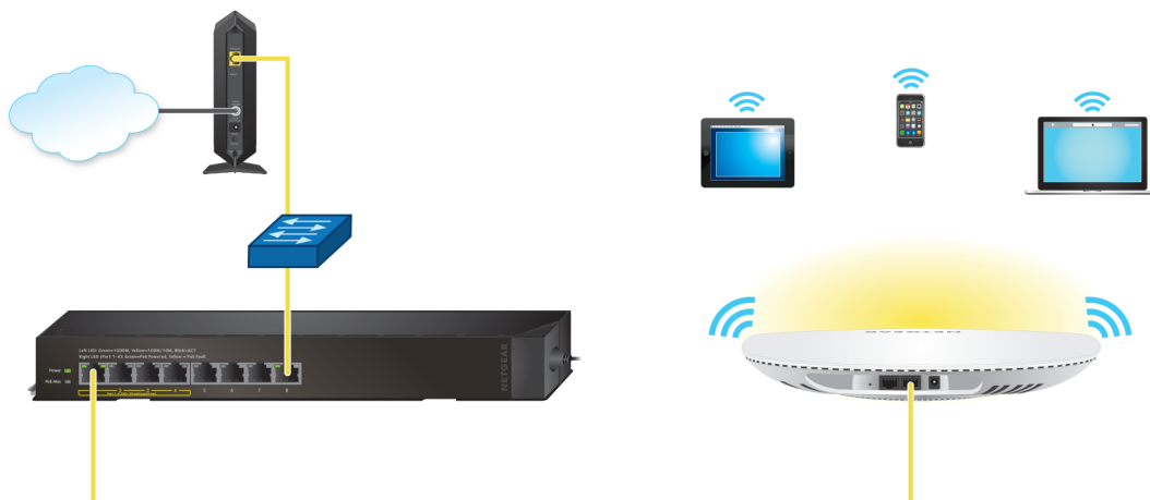
Figure 4. Set up the access point with a PoE+ connection to your network
