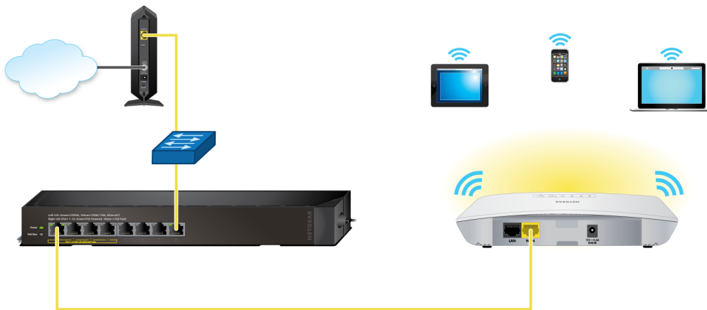
Figure 5. Set up the access point with a PoE connection to your network
