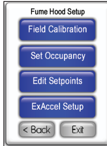
Figure 4. This menu provides options for recalibrating the sidewall sensor and sash position sensor, as well as configuring the target setpoints for each operating mode.
