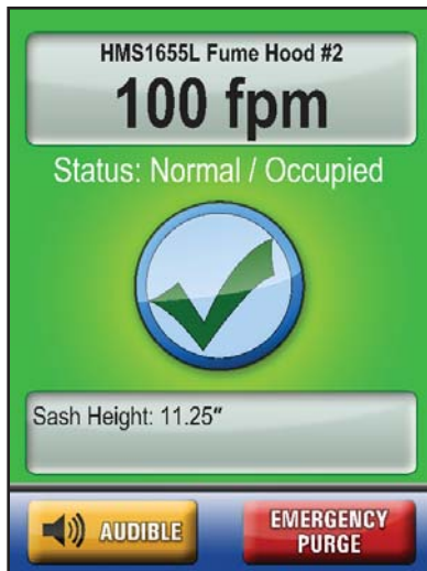
Figure 10. Tapping the Emergency Purge button instantly puts the fume hood in maximum face velocity mode.
