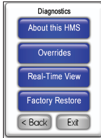
Figure 9. Built-in diagnostics may be accessed at this menu to assist with troubleshooting and initial setup of this controller.
