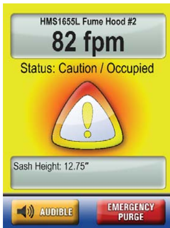
Figure 3. When the face velocity drifts outside the normal operating range, the main display background turns yellow to indicate a warning condition.
