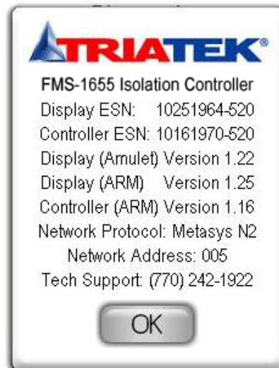
Figure 85. The About popup screen reveals pertinent information such as firmware versions, serial numbers, and network address.
