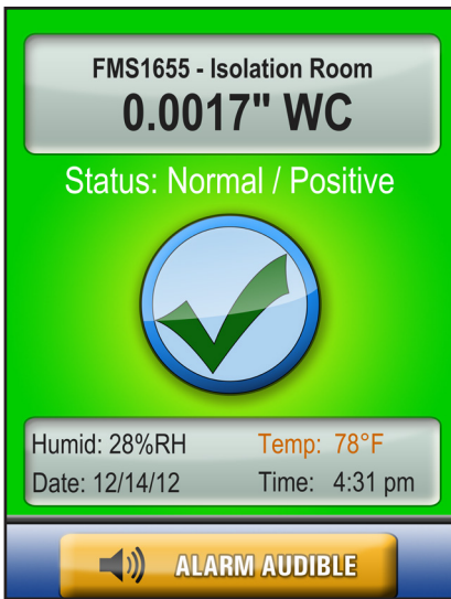
Figure 65. Temperature warning while in normal mode is represented by orange temperature display.
