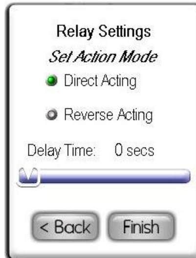
Figure 55. The action mode and delay time for secondary relays may be configured at this popup screen.
