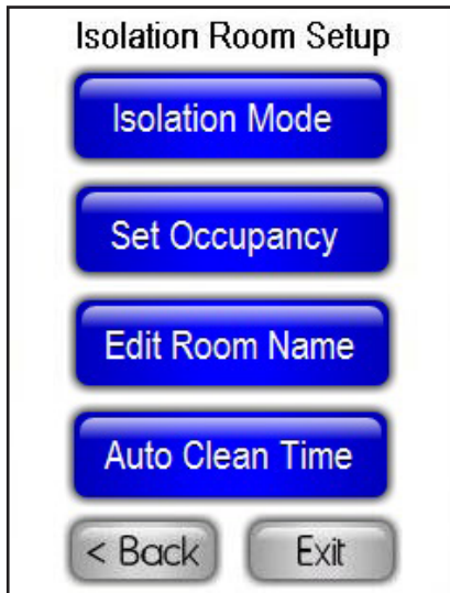
Figure 23. Settings specific to the space being monitored and/or controlled may be configured at this menu. The time duration associated with the automated clean cycle may be configured from this menu.
