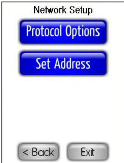
Figure 28. Network Setup menu options available for units configured for Metasys N2 protocol.
