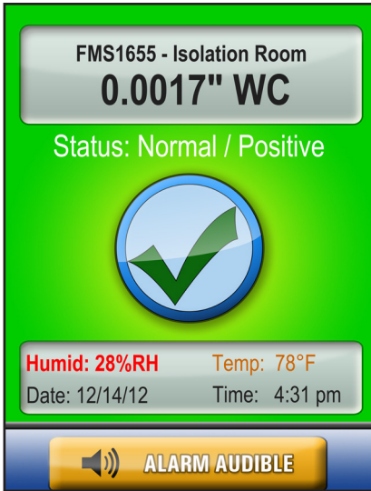
Figure 64. Humidity alarm and temperature warning while in normal mode is represented by red and orange displays, respectively.
