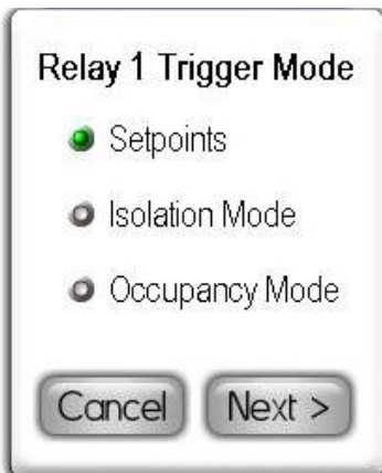
Figure 13. Relays may be triggered by one of three methods, and may include an activation delay.
