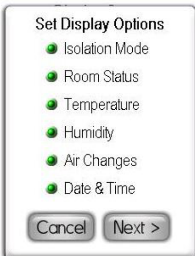
Figure 75. This configuration popup allows the main display to be customized based on the parameters being monitored.
