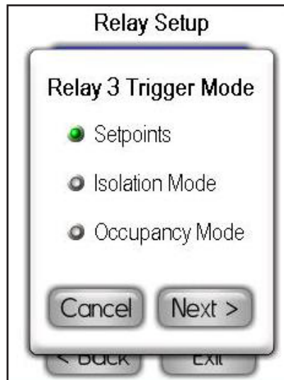
Figure 56. Secondary relay outputs may be triggered in one of three modes, with the default being Setpoints mode.
