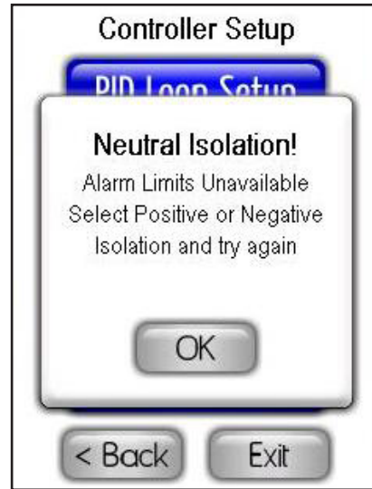
Figure 17. Positive or negative isolation mode must be currently active to enter alarm setpoints. Otherwise, this message is displayed.
