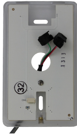
Fig 2. Route interface cable through center hold at display enclosure backplate.
