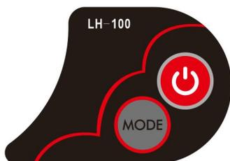
1. When it is shutdown, long-time pressing
