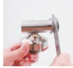
2. Spear Cross-Bar Leakage Solution: There is Nut Under Spear Body, tighten the Nut to prevent by Tool.
