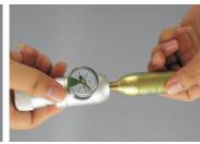
6, Turn in a new 16g CO2 capsule with thread type of 3/8"-24 UNF, turn clockwise firmly into the regulator base. Important: DON'T stop turning if you hear a slight gas leak swish, finish turning it in all the way it seal properly.
