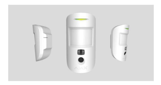
**MotionCam** is a wireless motion detector with visual alarm verification for indoor use. It operates for up to 4 years on bundled batteries, detects movement at up to 12 meters, ignores animals, but recognizes a human move instantly. MotionCam works within Ajax security systems, connecting to a hub through the two secure radio protocols. The detector uses Jeweller to transmit alarms and events, and Wings to transmit photos. Wireless coverage may reach up 1,700 m line-of-sight.
