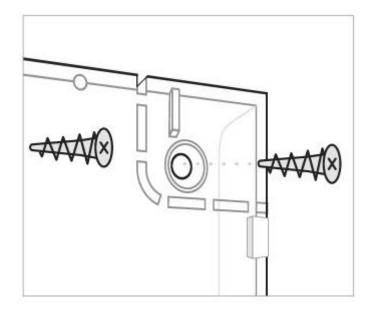
2. Attach the detector to the mounting panel. As soon the detector is fixed in SmartBracket, its LED blinks once to signal that the tamper on the detector has been triggered.
