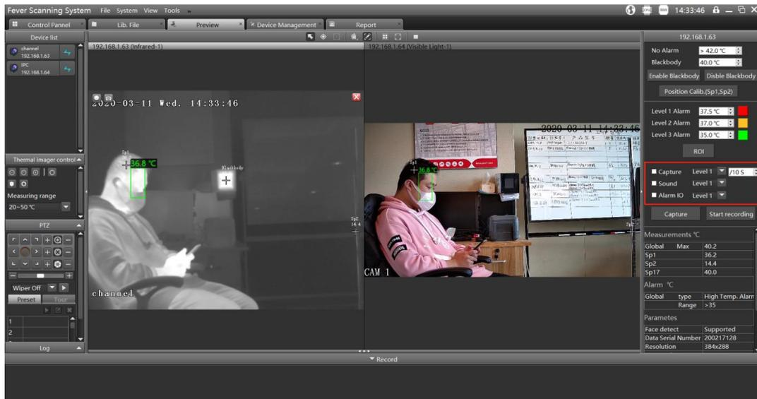
Figure 10 Alarm event (image capture and sound alarm)
