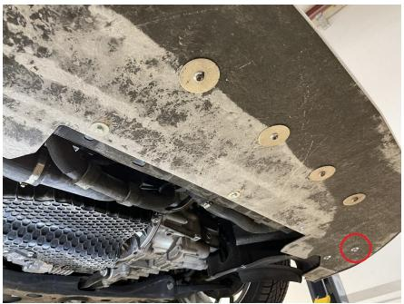
17.) Check that all bolts and screws are secure. It is important that the rods are fully tightened.
