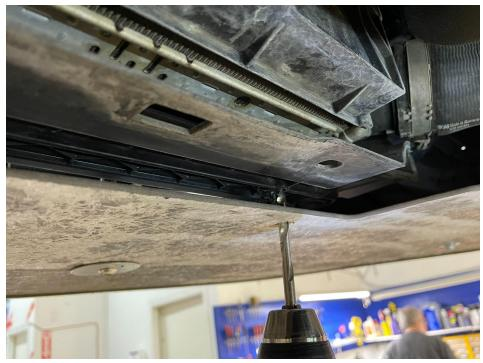
10.) Make sure your rods are fully closed and install the splitter onto the bottom of the rods with loctite. Use the  $\frac{3}{4}$ " wrench to hold the rod ends. Use  $\frac{5}{16}$ "-18 x 0.75" button head bolts and the 1.25" OD washers. This will be tricky. Use help to support the splitter - as a shop ourselves we use a table in conjunction with a lift.
