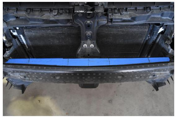
6.) Drill 5/16" holes at those 4 locations. Pass through both the top and bottom of the crash bar.
