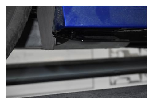
4. Install one of the T25 bolts you just removed into the second hole in the skirt/rockerpanel from the rear. Install the shorter (1") body screw into the 3rd hole from the rear with a 5mm spacer in between the side skirt and rocker panel. Again don't tighten much, only use them as points to hold up the skirt.
