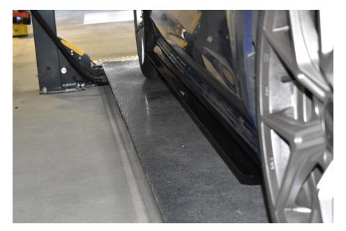
5. Identify where double sided tape is needed under the rocker panel based on where the skirt sits. Remove the side skirt, clean the underside of the rocker panel, and apply heavy duty double-sided tape to the rocker panel. We placed 2" wide tape in the areas that had little body screw support. We also added <u>a lot more</u> than what is seen in the pictures for extra support and we recommend you do as well (it was an afterthought)!
