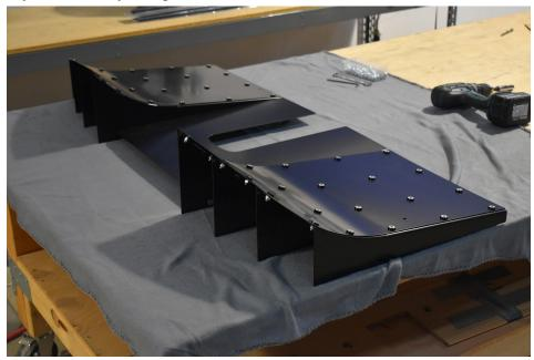
7.) Needed: (4) M6-1.0 x 20mm bolts, (4) 1" OD fender washers, (4) ½" small washers, (4) M6 nyloc nuts. With help from a friend install the diffuser onto the steel brackets pointing the bolts upward. Use the fender washers on bottom. Use the small washers and nyloc nuts on top. Securely tighten.
