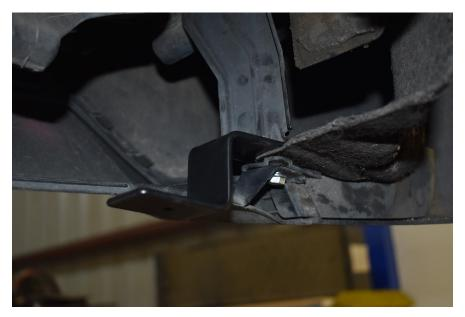
5.) Remove the two T25 screws toward the center of the car on either side of the exit tips. You'll be using the built-in clips so don't even think about removing those. :)
