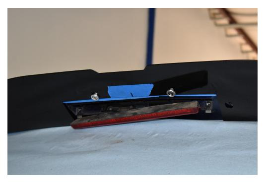
9. Push the spoiler extension up against the OEM spoiler and mark the outer two holes with your sharpie then remove the spoiler extension. Drill holes into these marked locations. Start with an ½" (or small bit) to center the hole then move up to a ½" hole. Our transition went like this: ½", ½", ½". Having drill bits that have tapered ends <u>really</u> helps. Be careful with the ½" and TAKE YOUR TIME. This is a fairly large hole!
