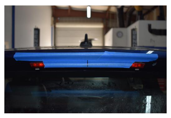
4. Apply painter's tape to the center of the spoiler extension on the side that faces toward the back of the car. The backside of the spoiler extension is the side that has the washer fluid hole on the right. Mark the center of the spoiler extension with your marker on the painter's tape.
