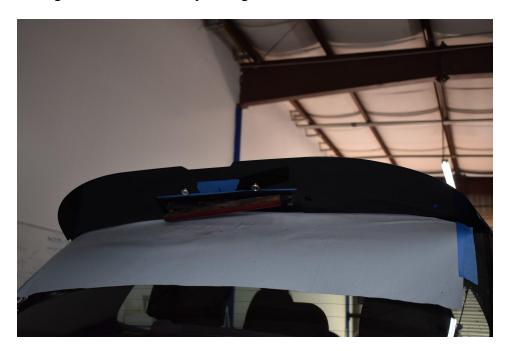
2. Apply painter's tape to the back side of the car's OEM spoiler. Cover the areas shown in the picture including some of the 3rd brake light.
