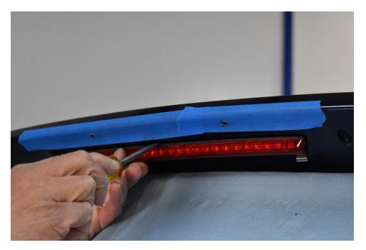
8. Install the spoiler extension onto the car using only the two center holes. Use your M6 bolts and nuts, and your washers. The nuts will sit on the inside of the OEM spoiler (this is a bit tricky to install, have a friend with skinny fingers help). Hand tighten. Feel free to leave the tape on as you will be removing the spoiler extension later.
