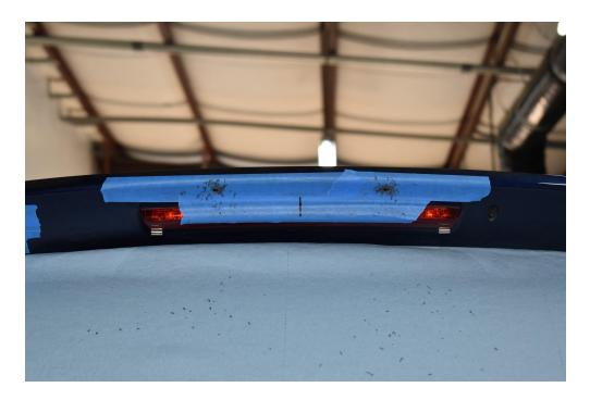
7. Remove the tape over the 3rd brake light. Remove the 3rd brake light. This can be done by first using your flat head screwdriver to push down the silver tabs found on each side of the 3rd brake light, then using the screwdriver to push the top center of the brake light down (2 pics).
