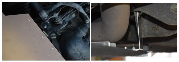
5.) Now, install the front end of the rearward underbody panel onto the chassis bracing. There will be one hole in the center of it that matches up to the panel. Use a M6-1.0 x 30mm bolt pointing upward - 15mm spacer in between, 1" OD fender washer on bottom, M6 nyloc nut on top. Securely tighten.
