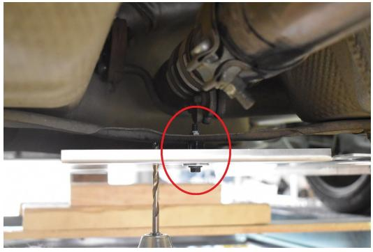
6.) There are holes in the rearward panel on either side of the hole from the previous step. Drill through those holes into the chassis bracing with a ¼" diameter drill bit. BE SURE TO DRILL STRAIGHT UP & feel free to start with a little bit first to align the hole. Then, install the same bolt/washer/spacer/nut combination into the holes just drilled. You might have to loosen the
