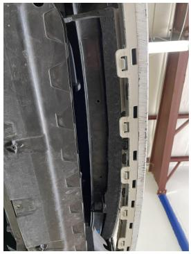
9.) Make sure the holes you drilled are clean on top and bottom. Drop down the splitter rod's FOUR 5/16"-18 x 1" hex bolts with 1.25" OD washers into the holes just drilled.
