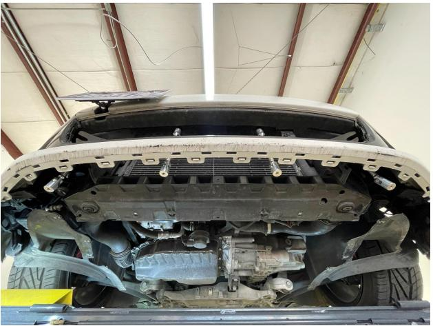
12.) Now identify and drill out the radiator support mounting locations with a  $\frac{1}{4}$ " drill bit. There are four. Make sure the drill doesn't push through and hit a hose above.
