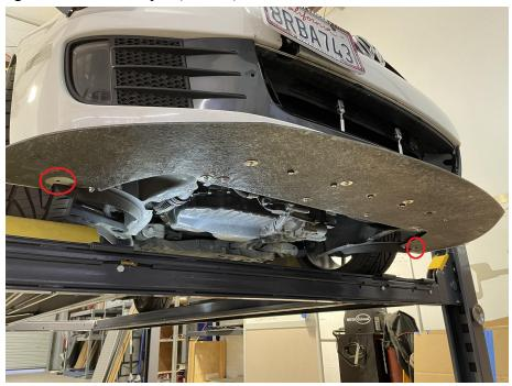
17.) Install your splitter into the holes where the OEM brake ducts are held. Use four M6-1.0 x 30mm bolts with 15mm spacers between the splitter and locations (2 spots on each side). You will need to remove the OEM speed nuts. Use 1.25" washers on bottom, and  $\frac{1}{4}$ " small stainless washers and m6 nyloc nuts on top.
