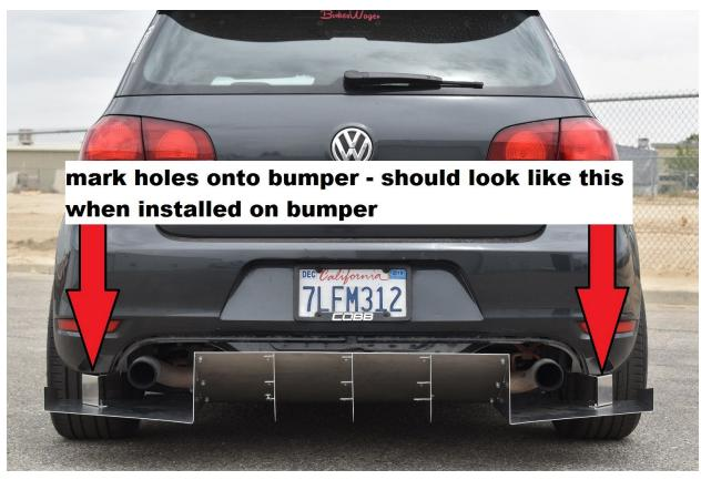
10. Remove the outer diffuser pieces and drill the holes you just marked on the bumper. Use your drill and  $\frac{1}{4}$ " diameter drill bit. (1 PIC)
