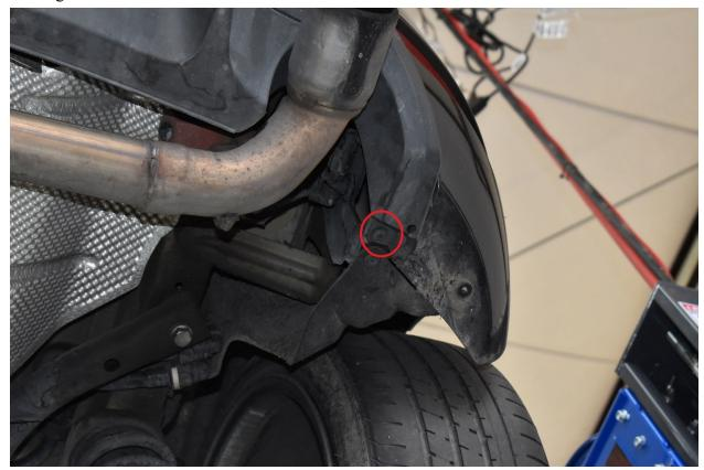
3. Remove the rear valence by pulling it away from the car. Feel free to use a flat head screwdriver to help pry the tabs away from the bumper. (3 PICS)
