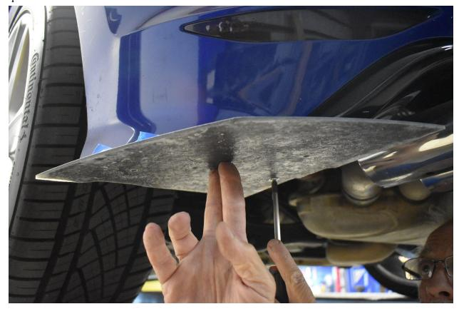
6.) Align the spat with the rear edge of the fender well. Then mark the holes in the spat onto the bumper.
