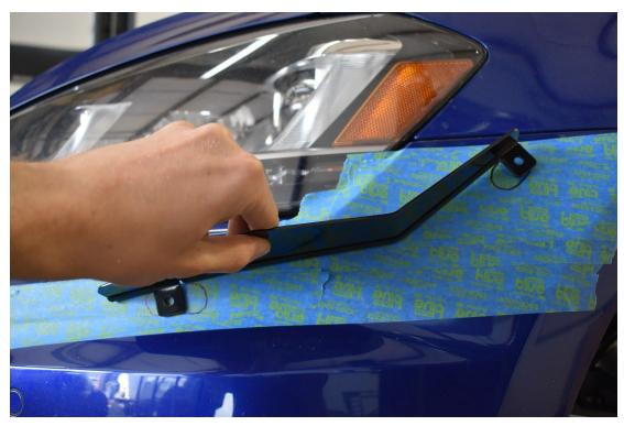
5. Hold the canard up to the car and make a mark through the mounting tab toward the front of the car. Drill a ¼" diameter hole and temporarily mount your canard with a bolt + WIZNUT. The wiznut is provided so you can easily add or remove the bolt. Install your canard into the single hole then use it to locate the ¼" diameter for the second hole. Drill that hole. (2 pictures)
