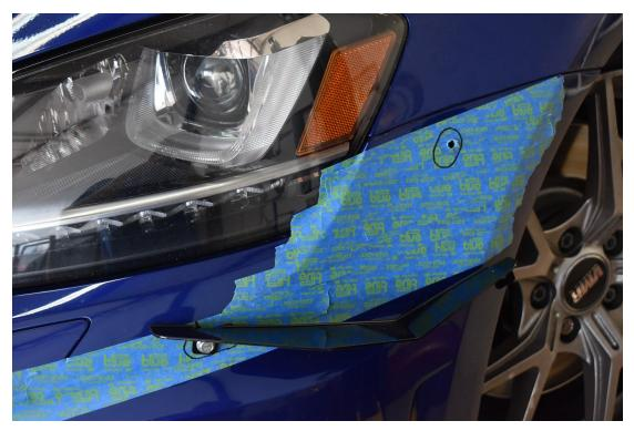
6. Remove the tape and install the canard onto the car. Slip the bolts through the mounting tabs and place a rubber washer between the canard and body of the car. On the inside of the bumper use a washer and nyloc nut to the secure the bolts. DO NOT overtighten. You are tightening onto plastic and there isn't much need to go all out. A 10mm wrench should be used on the inside and a 10mm socket + ratchet on the outside. (3 pictures)
