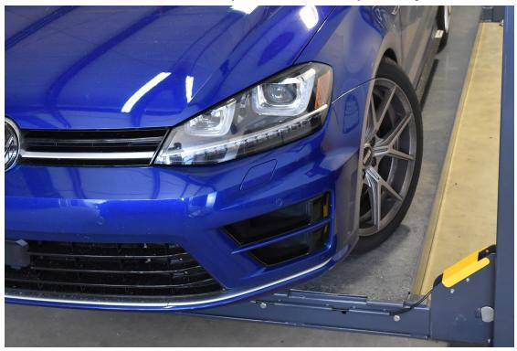
2. Apply painter's tape to the bumper where the canard will mount. We applied 4 layers of tape to protect the paint.
