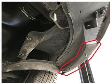
7. Test fit the splitter onto the steel brackets using 5 medium length bolts (facing up or down) and corresponding nuts. Allow the splitter holes to slide over the longer bolts installed in step (5.). Use nuts on these longer bolts to hold up the diffuser. Center the diffuser best as possible and with your sharpie mark the 2 holes on either side of the splitter on the blue tape (indicated in following illustration).
