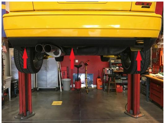
3. Hold the diffuser in place aligning the holes in the diffuser with the holes in the rear bumper. This might be easier with help from a friend. Install the supplied bolts and washers to hold the diffuser to the car, but do not tighten at this time.
