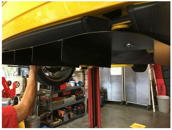
4. Align the diffuser so that it is even on each end of the bumper. Tighten the bolts (no torque specification but do not overtighten) and adjust as necessary (optional: green or blue thread locker – results in more removal).
