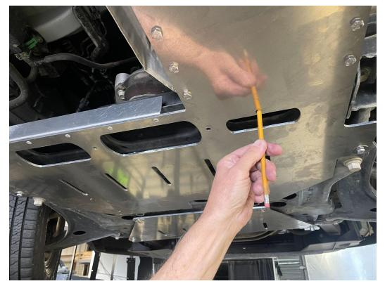
10.) Remove the guard and drill  $\frac{3}{8}$ " holes through the frame where the three holes were marked. **ONE:**
