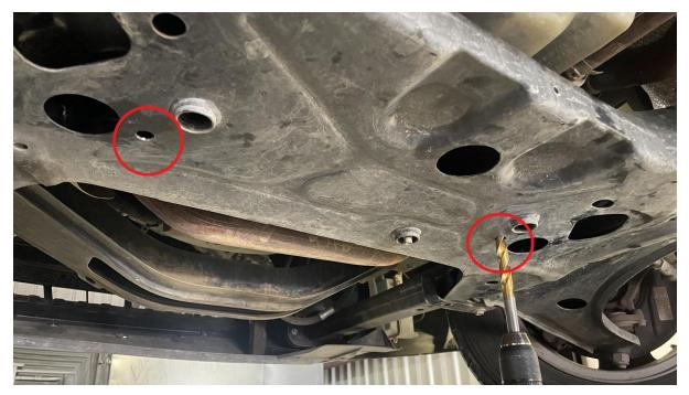
7.) The front cat guard can now be installed. The forward two OEM threaded holes use the M8-1.25 x 40mm hex bolts + washers. Use blue threadlocker on the threads.
