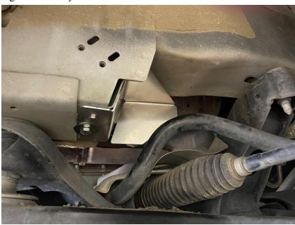
4.) Let's install the front guard. Remove the two bolts shown in the frame using a 13mm wrench. These are found under the engine. Don't remove the outer bolts.
