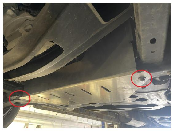
6.) Mark the two holes in the front guard onto the frame, then remove the guard and drill 3/8" holes where you marked.
