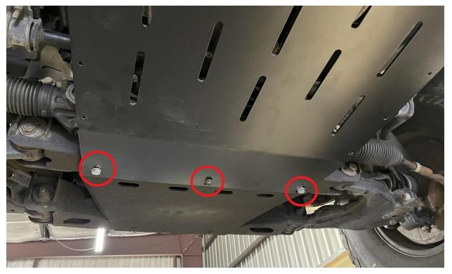
9.) Install your side plates - there is a left and right (see pics). Use the  $\frac{1}{4}$ "-20 x 1" long security bolts. Be sure to apply blue threadlocker on the threads when installing. A  $\frac{1}{4}$ " socket will be necessary for the security bit. No need to overtighten here.
